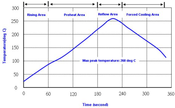
Note: 1.Max peak temperature: 260+/-5 deg C; Time: 10+/-2 sec 2. Temperature: 217+/-5 deg C; Time: 90~100 sec TAI-SAW TECHNOLOGY CO., LTD. TST DCC Release document
